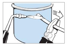
Figure 26.b - Separating the compressor from the system's tubes
