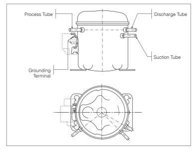
Figure 34 - PW compressor with copper tubes
