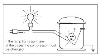
Figure 24 - PW/F/EG Compressor Coil Test
