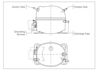
Figure 30 - EM Compressor with copper tubes
