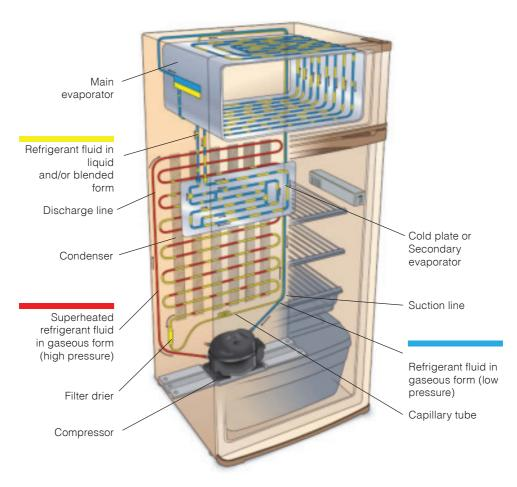
Figure 1 - Operation of a basic refrigeration system
