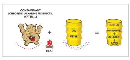
Figure 41 - R 134a chemical reaction between contaminants and ester oil
