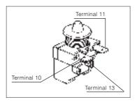
Figure 37 - Short relay without capacitor
