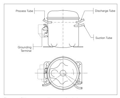
Figure 35 - PW compressor with copper-plated tubes
