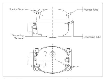
Figure 31 - EM compressor with copper-plated steel tubes
