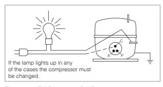
Figure 24.a - EM Compressor Coil Test
