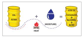
Figure 42 - Chemical reaction between ester oil and water
