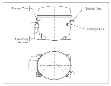
Figure 32 - F/EG compressor with copper tubes
