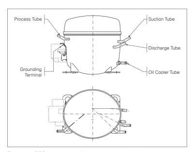
Figure 33 - F/EG compressor with copper-plated steel tubes
