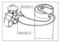
Figure 38 - Short relay with capacitor
