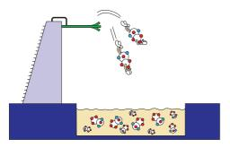
Ester oils have been specially developed to work with R 134a (acceptable miscibility).
