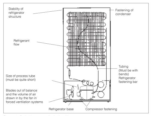
Figure 21 - Probable sources of noise in refrigerators
