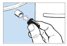
Figure 26.c - Closing the tubes with rubber plugs
