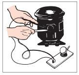
If the lamp goes on the main coil is not broken.
