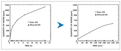
Figure 43 - Graphs comparing hygroscopicity between ester oil and mineral oil
